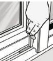
**EN:** Remove the transport blocks and open the centre mullion lock. Take away the aluminium strip under the sliding leaf
