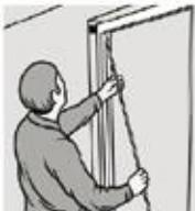
**EN:** Side jambs must be adjusted to be vertical and in plane and all diagonals
