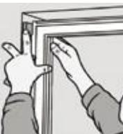
**EN:** Position the frame in the predetermined place and wedge the fixed part first with temporary wedges (opposing wedges from inside and outside), then the opening side at all 4 corners.
