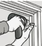
**EN:** Place exactly fitting blocks where the windows fixing holes are positioned, and fix with screws where the predrilled holes are positioned in the frame.
